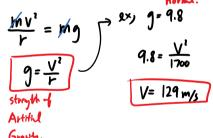
5. (Space: Artificial G) A space laboratory is rotating to create artificial gravity. Its period is chosen so that the outer ring (r = 2150 m) simulates the acceleration due to gravity on Earth. What should the radius of the inner ring be so that it simulates the acceleration due to gravity on the surface of
