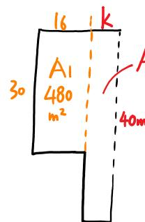
$$\begin{aligned} \text{half Room} &= A_1 + A_2 \\ 600 &= 480 + 40k \\ 120 &= 40k \\ k &= 3 \text{ m} \end{aligned}$$
