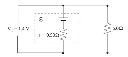
$I = \frac{1.4 \text{ V}}{5.0 \Omega} = 0.28 \text{ A} \quad \leftarrow 1 \text{ mark}$
