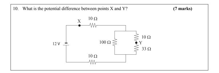
$$R_{T} = 10\Omega + 10\Omega + \left(\frac{1}{100\Omega} + \frac{1}{(10\Omega + 33\Omega)}\right)^{-1}$$
