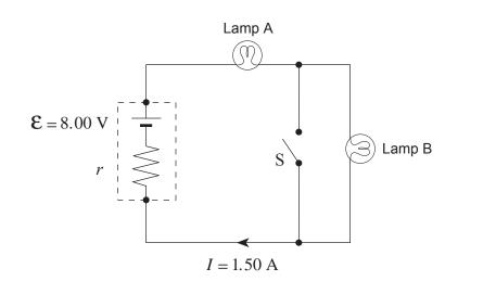
a) If a current of 1.50 A flows in the circuit, what is the internal resistance r of the battery? (4 marks)
