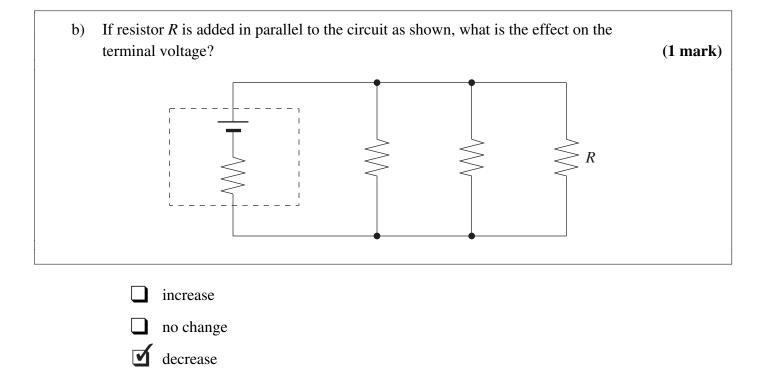
Additional *R* in parallel results in an overall lower *R*, thus an increase in current. (2 marks) As a consequence, a greater voltage drop *Ir* occurs across the internal resistance resulting in a smaller terminal voltage. (2 marks) 2. Consider the circuit shown in the diagram below.
