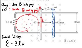
$\xi = 0.33 (0.3 \text{m})(6.2) = 0.6138 \text{ V}$  $V = IR \qquad I = \frac{V}{R} = \frac{0.6138}{9} = 0.068 \text{ A}$  4. A single loop of wire encloses an area of 0.035m<sup>2</sup>. The magnetic field changes in a time of 0.060s. What is the induced emf and direction of the current flow in the loop? (0.57V, counterclockwise)
