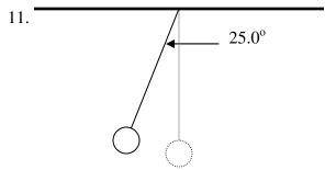
A pendulum is 1.20 m long. If the pendulum is pulled until it makes a  $25.0^{\circ}$  angle to the vertical, what is the speed of the pendulum bob when it passes through its equilibrium position? HINT: Determine the vertical drop of the pendulum bob first. 1. How much heat is needed to rise the temperature of 462 g of water from 24.0  $^{\rm o}{\rm C}$  to 80.0  $^{\rm o}{\rm C}?$
