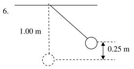
A pendulum is dropped from the position shown, 0.25 B m above its equilibrium position. What is the speed of the pendulum bob as it passes through its equilibrium position?
