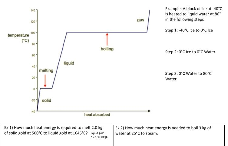
Ex 3) How much heat does a refrigerator freezer have to remove from 1.5 kg of water at 20°C to make ice at -10°C
