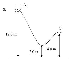
A roller coaster car starts from rest at point A. What is its speed at point C if the track is frictionless?
