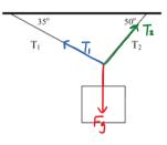
An object is suspended as shown. If the tension in one of the ropes is 50 N as shown, what is the weight of the object?
