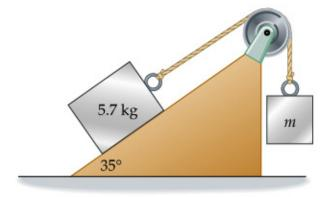
6. Find the tension in the connecting rope above once the blocks have moved 30 cm. (ans: 56.4 N)
