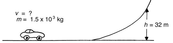
If the car comes to a stop when it reaches a vertical height of 32 m, what is the minimum speed it must have had when it entered the runaway lane? (ans: 25 m/s)
