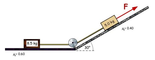
8. Determine the applied force **F** that would accelerate 5.0 kg block above up the incline at 2.5 m/s<sup>2</sup> (ans: 125.2 N)
