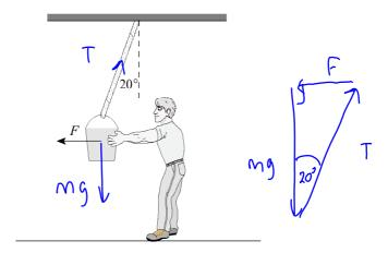
a) Find the tension force in the supporting rope.
