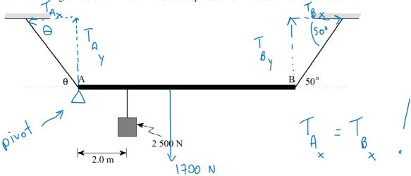
Determine the tension in the cord attached at end A and the angle  $\theta$  that the cord makes with the horizontal. (diagram is not to scale) (10 marks)
