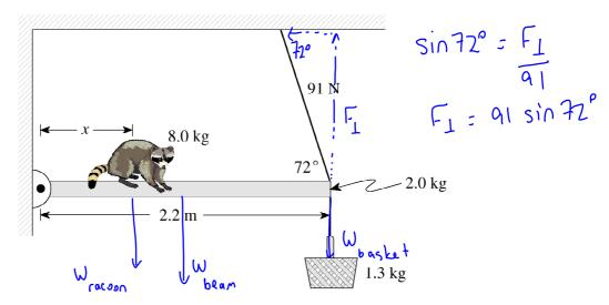
What is the maximum distance, x, the raccoon can walk out onto the beam before the cord breaks?
