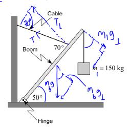
What is the tension in this cable when the boom supports a 150 kg mass as shown? (7 marks)
