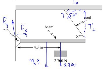
a) Draw a free-body diagram that identifies the forces acting on the beam.
