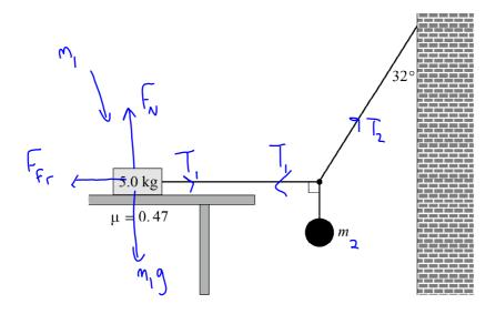
A coefficient of friction of 0.47 exists between the 5.0 kg block and the table. What is the maximum mass, m, that can be hung from the cords before the 5.0 kg block begins to move?
