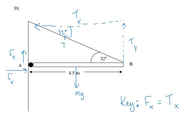
The above diagram shows a uniform 24 kg beam hinged to the wall at A and supported at B by a cable. What is the magnitude of the **horizontal** force exerted by the wall on the beam? (10 marks)
