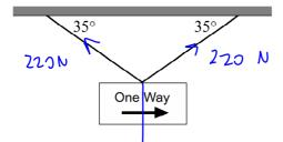
If the tension in each cable is 220 N, what is the weight of the sign?
