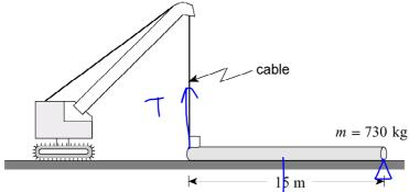
What is the minimum force of tension in the crane cable to just lift the end of the pipe off the ground?
