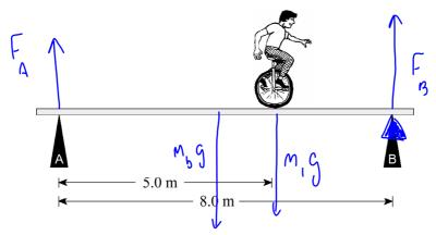
a) When he is at the position shown, determine the forces exerted by the supports on the
