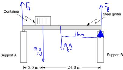
What are the upward forces at the girder end points when it is bearing a 3 700 kg shipping container 8.0 m from support A? (7 marks)
