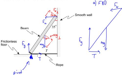
a) Draw a labelled free-body diagram for the forces acting on the beam.
