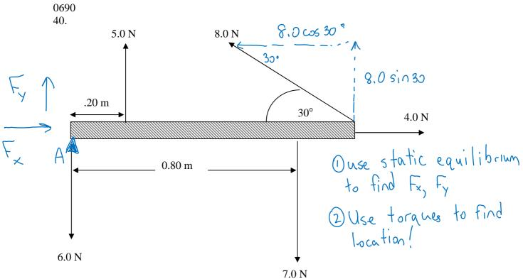
A bar 1.0 m long has five forces acting on it as shown in the above diagram. What are the **magnitude**, **direction**, and **location** of the single force required to produce static equilibrium? The weight and thickness of the bar are insignificant. (12 marks)
