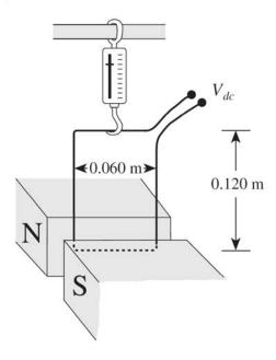
As the current in the loop is varied, the readings of the spring scale and current are plotted on a graph.
