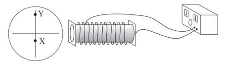
What changes to the magnitude and direction of the current in the solenoid would cause the electron beam to strike the screen at Y?
