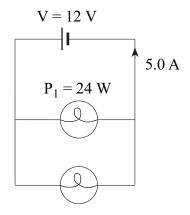
The power output of one of the bulbs is  $P_1 = 24$  W. What is the power output of the other bulb?
