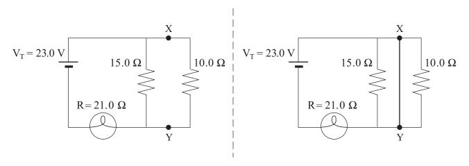
What is the current through the light bulb and what happens to the brightness of the bulb when the wire is connected?
