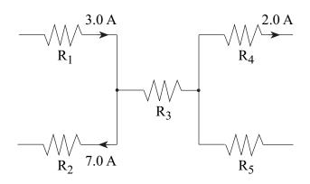
What are the magnitude and direction of the current passing through resistor  $R_5$ ?
