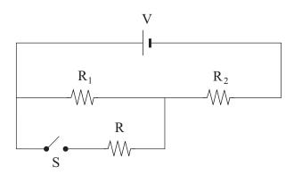
How does the current through resistors  $\mathbf{R}_1$  and  $\mathbf{R}_2$  change when switch S is closed?
